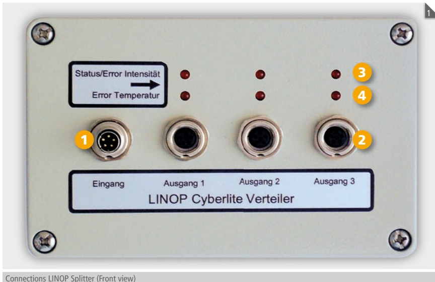
Connections LINOP Splitter (Front view)
