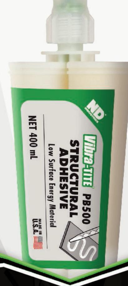
2-part methacrylate based adhesive that is specially formulated to bond low surface energy materials such as polypropylene, polyethylene and PTFE without additional surface preparation. The PB500 offers increased working time while also building ultimate strength faster than other adhesives in its class. The PB500 material offers high impact resistance and is capable of withstanding extreme temperature fluctuations.
